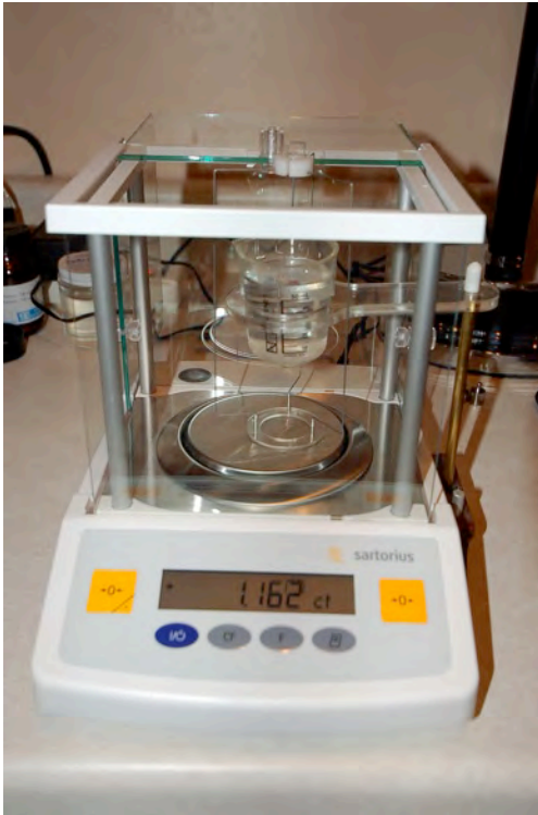
A Sartorius gem balance with specific gravity attachment
