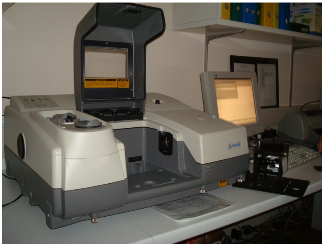
A Fourier Transform Infrared Spectrophotometer in use at the SSEF in Basel, Switzerland.
