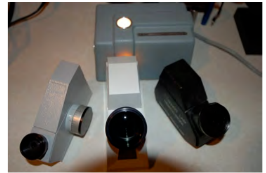
A lightsource with monochromatic filter and refractometers, a Dialdex, Duplex II and Gem Pro
