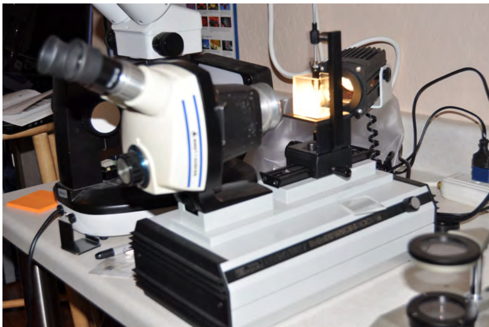
An Eickhorst horizontal microscope base designed for immersion and polarization work. The base is fitted with a B&L Stereozoom 5 head.
