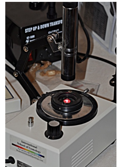
The ISG sells a small light base with rheostat and iris diaphragm with a generic prism spectroscope for about $450.
