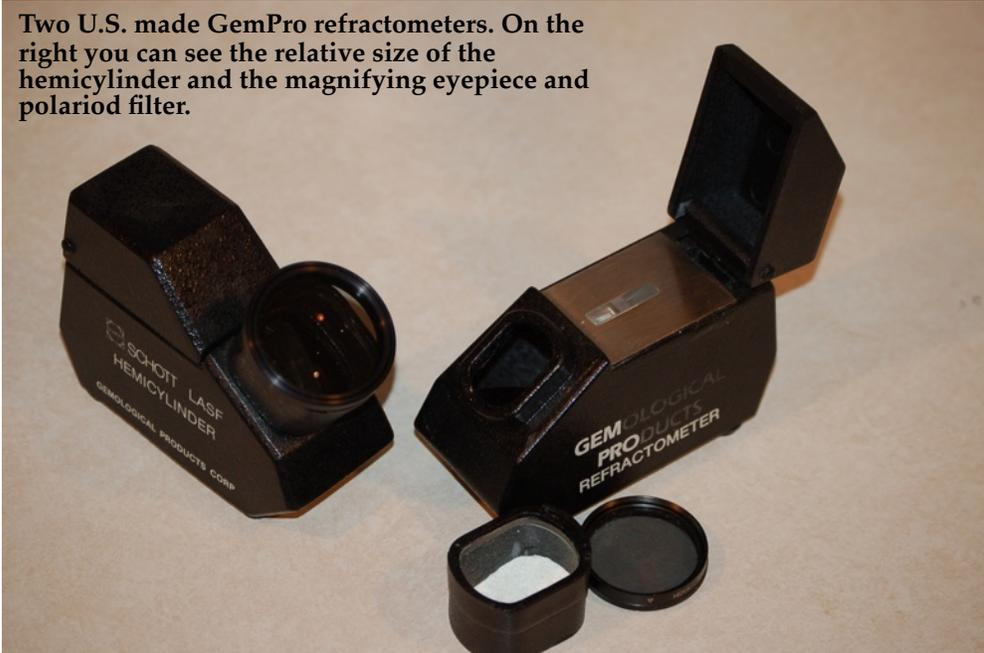
Two U.S. made GemPro refractometers. On the right you can see the relative size of the hemicylinder and the magnifying eyepiece and polaroid filter.
