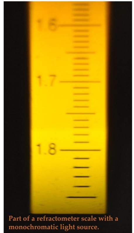
Part of a refractometer scale with a monochromatic light source.
