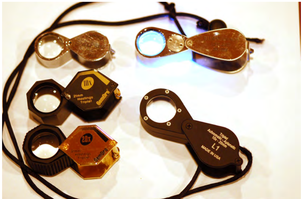
The loupe in the top left is a Bausch & Lomb that has served for 30 years. You can buy one today for less than $35. Center left is a Gem Oro 10x loupe followed by a Gem Oro 20x loupe that while advertised as a triplet suffers from substantive spherical aberration. Upper right is generic Chinese loupe with built in LED light. Bottom right is a GemologyPro Harald Schneider unit that is the highest quality 10x Achromatic-Aplanatic Triplet and costs $300.
