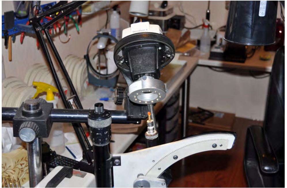
A B&L Stereozoom microscope with fiber optic ring-light is mounted on a boom and stand that allows direct observation of a stone on the dop of a GMII.
