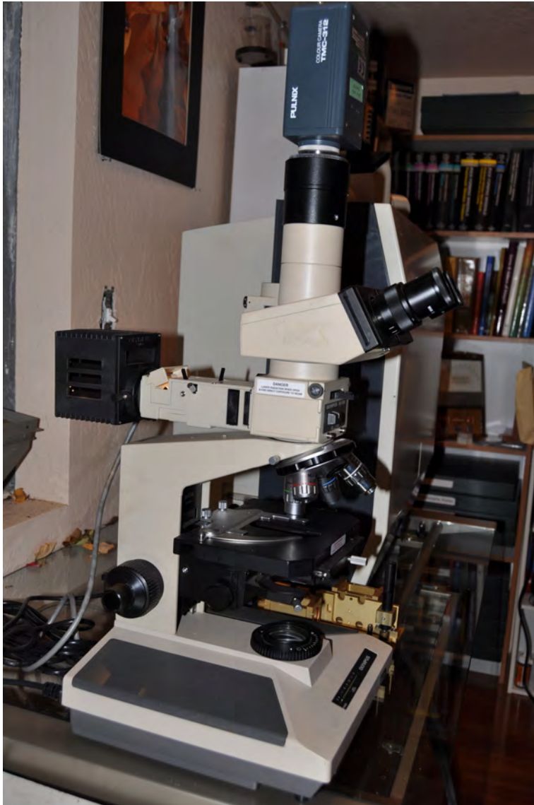
An Olympus BH-2 series set up for Raman microanalysis where laser light travels through the optic train and the objective lenses directly impinging on the sample at a 90° angle. The Renishaw Raman system is confocal and can identify virtually any organic or inorganic substance.
