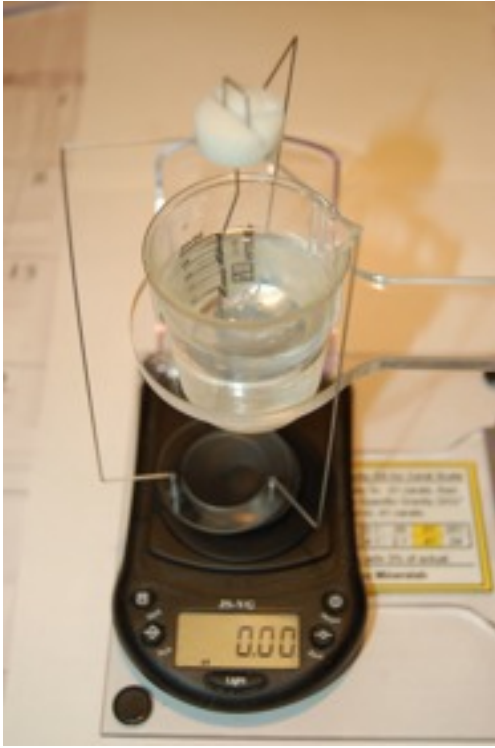
Step 2: Set up the S.G. kit on the scale and tare the scale so it reads zero.
