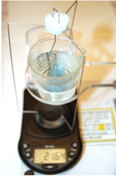
Step 3: Carefully place the stone on the wire holder in the water
