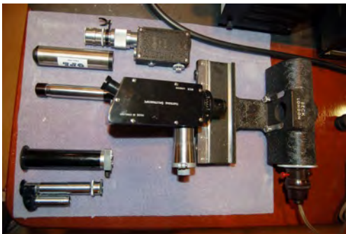
A series of spectroscopes, top to bottom: A Lafayette, an OPL, a generic prism, a Hartridge Reversion, a Beck and a Zeiss with wavelength scale
