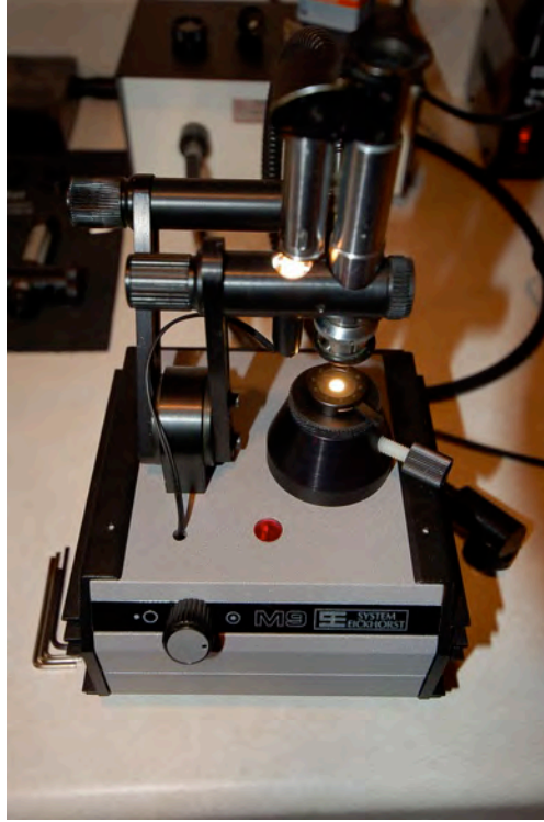
An Eickhorst M9 Spectroscope base fitted with a Zeiss prism spectroscope with scale
